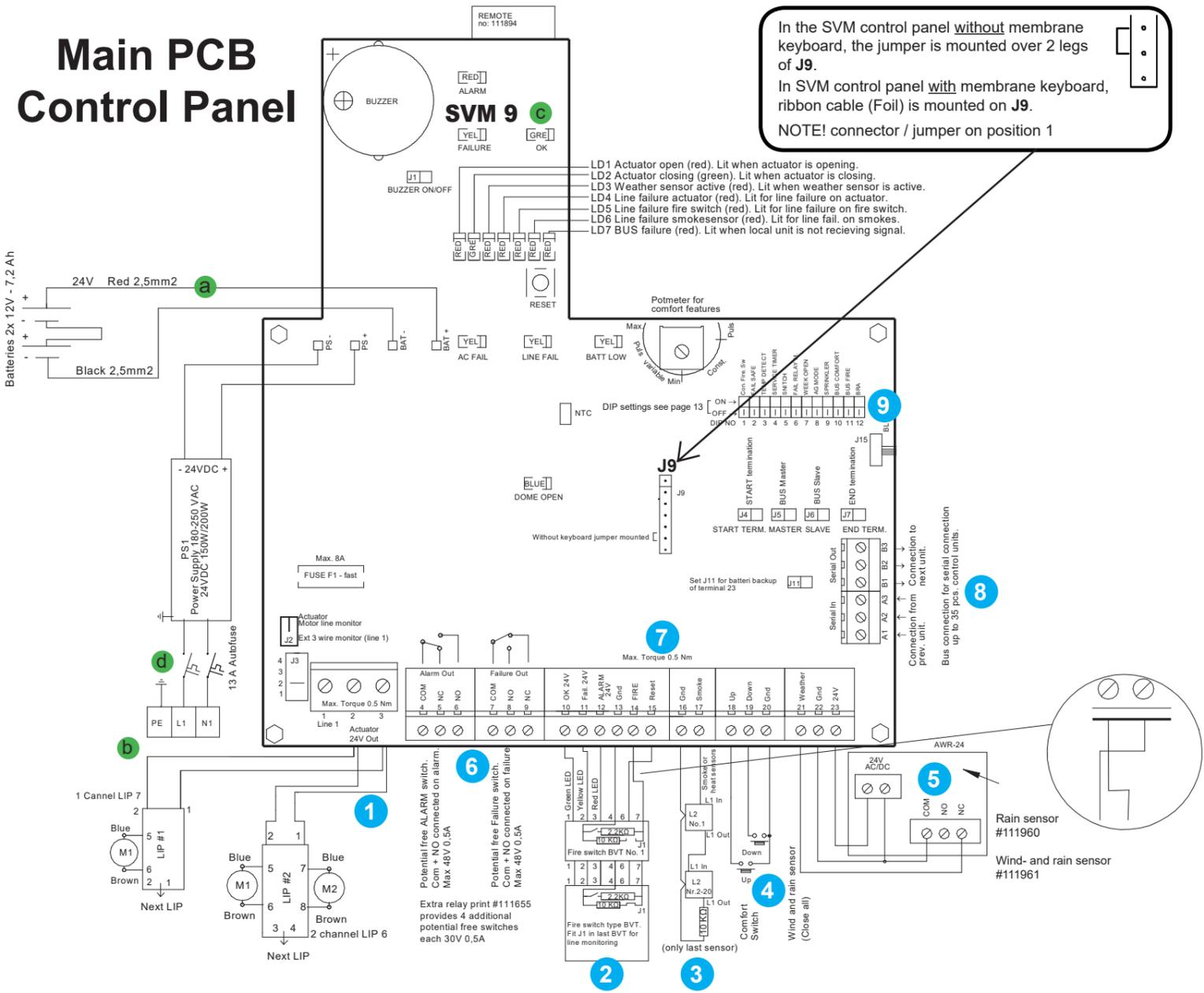
In the SVM control panel without membrane keyboard, the jumper is mounted over 2 legs of J9.
