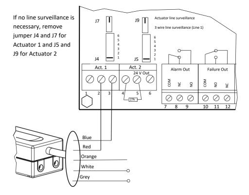
Caution: The white and grey core are only for changing parameters. Parameter change can only be made by Actulux or an authorized service and
