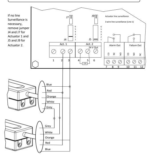
Caution: The white and grey core are only for changing parameters or for BUS communication in synchro mode. Parameter change can only be made by Actulux oran authorized service and sales partner by Actulux. Do not connect the white and grey wire to 24V!
