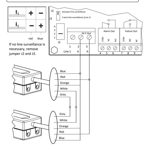
Caution: The white and grey core are only for changing parameters or for BUS communication in synchro mode. Parameter change can only be made by Actulux or an authorized service and sales partner by Actulux. Do not connect the white and grey wire to 24V!
