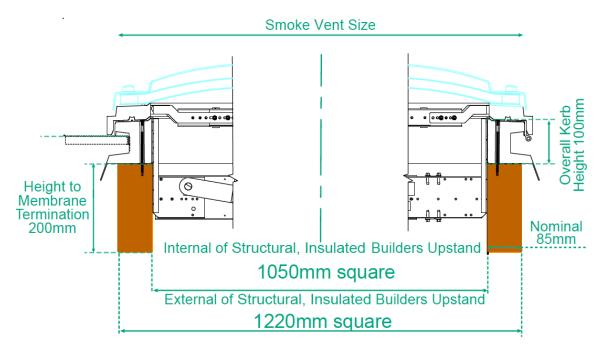
Smoke Vent Fixed to Structural, Insulated Builders Upstand
